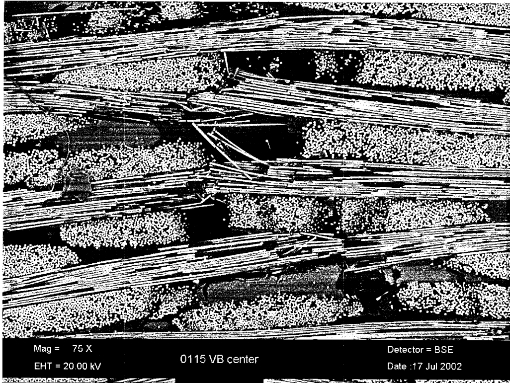
Figure 6-17 SEM micrograph of V/B 8/4 co-cured hybrid composite after flexural test – near the center of the specimen.
