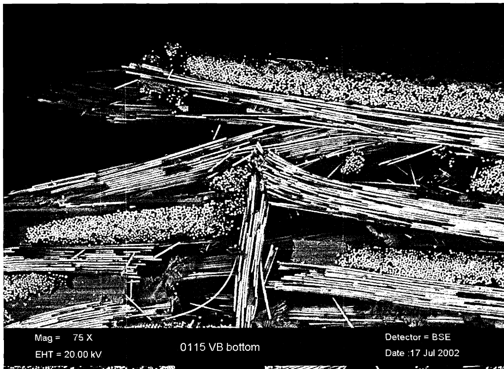
Figure 6-15 SEM micrograph of 2672B composite after flexural test.
