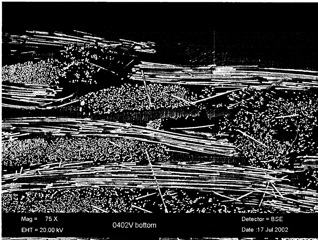
Figure 6-14 SEM micrograph of vinyl ester composite after flexural test.
