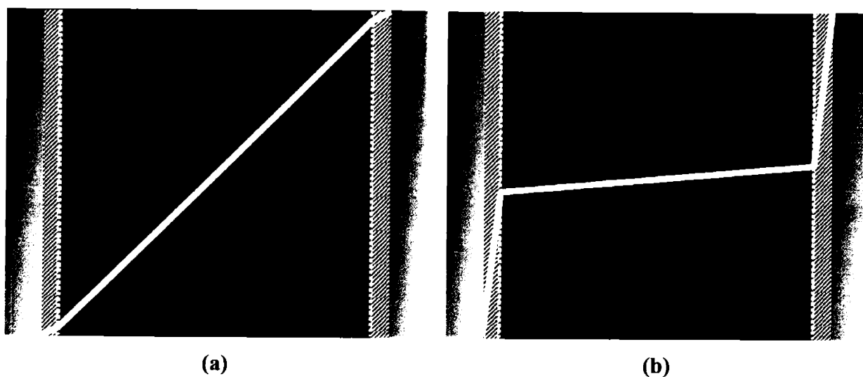
Figure 3.1: Schematic of (a) reversible and (b) blocking electrodes, showing potential drop as a function of position from the electrode-fluid interface.
