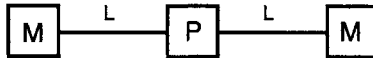
Figure 2-1: Schematic of long-distance quantum communication system. P = ultrabright narrowband source of polarization-entangled photon pairs; L = L km of standard telecommunications fiber; M = trapped-atom quantum memory.
