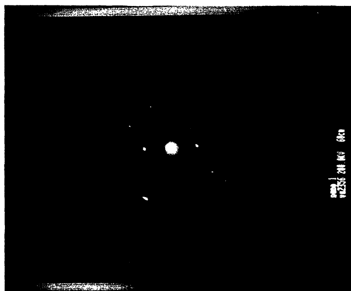
Figure 2.16: TEM Selective Area Diffraction (SAD) pattern of the core, showing that it is monocrystalline.
