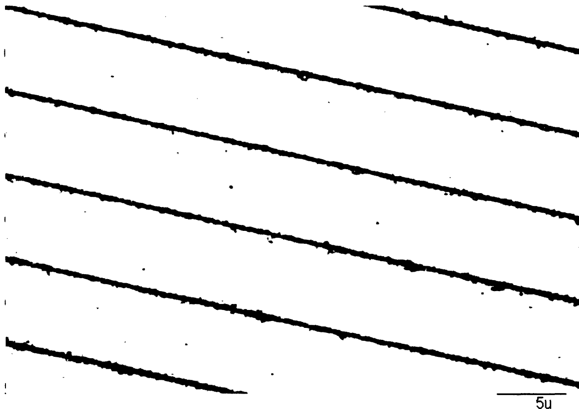
Figure 3.14: Optical micrograph of an electrified polyamide substrate decorated by pre-charged graphite nanoparticles dispersed in hexane.
