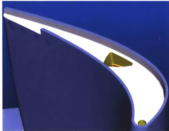
Figure F 3: Tip crown and internal cooling passage outlets.
