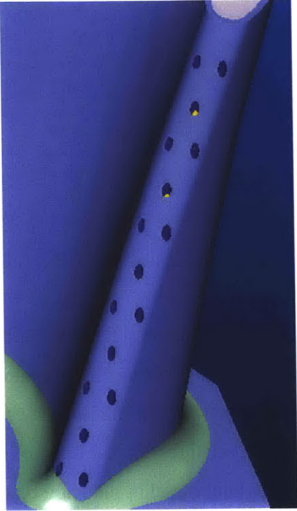
Figure F 4: Leading edge showerhead cooling configuration.
