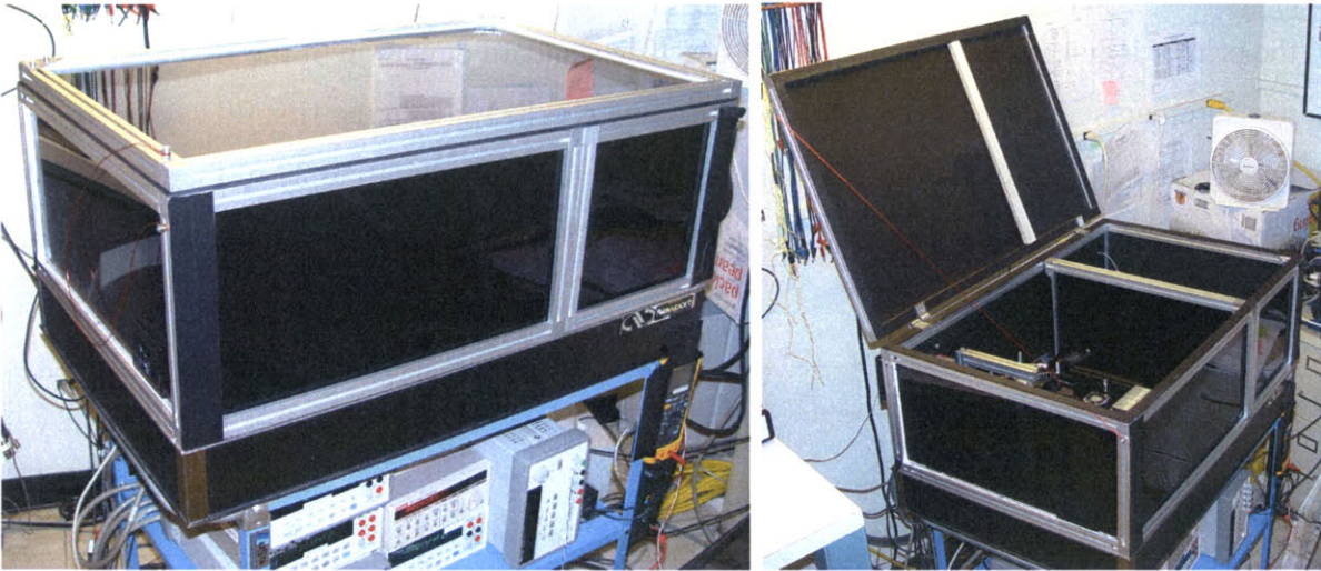
Figure 4-3. Instrument was housed in a light tight, temperature regulated enclosure consisting of two separate compartments.
