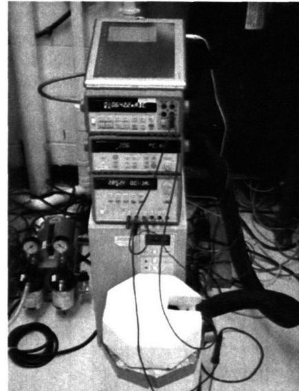
Figure 3: Scientific instruments controlled by tablet PC (from top to bottom: Agilent 34401A Digital Multimeter, Agilent 34970A Data Acquisition Switch with 34901A multiplexer card, and Agilent E3631A Power Supply).
