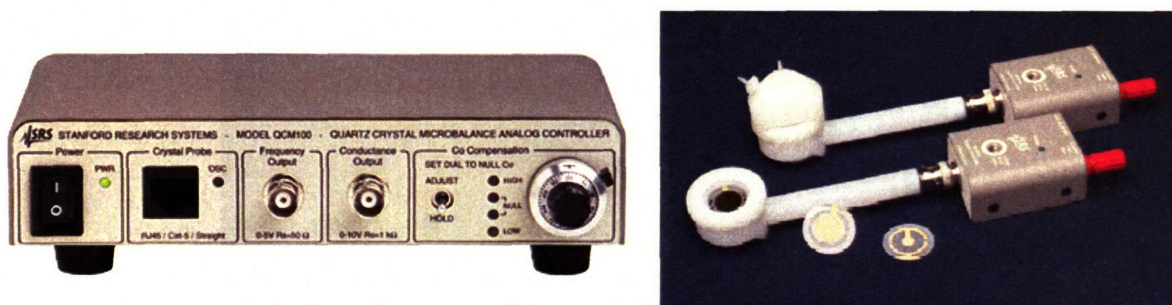
Figure 4.13: SRS QCM100 Quartz Crystal Microbalance control unit (left) and crystal holder (right) used to dynamically study mass transport to the working electrode. Source: http://www.srsys.com/
