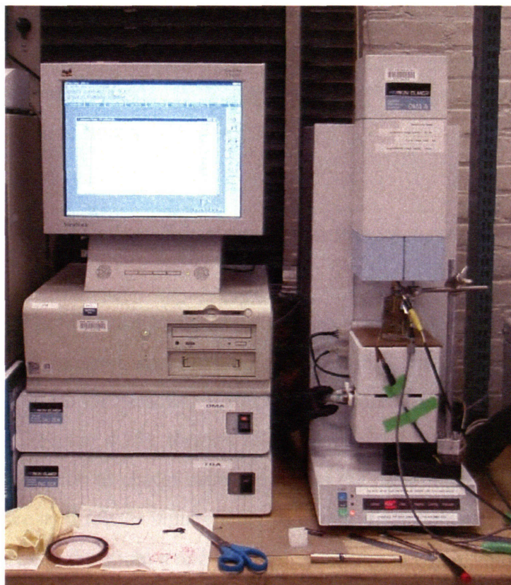
Figure 4.14: Photograph of the digitally controlled Perkin Elmer DMA 7e used in this thesis to characterize the passive properties of conducting polymer actuator films.
