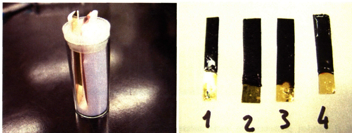
Figure 4.3: Electrochemical cell designed to handle disposable gold-coated PET electrode films (left) and resulting conducting polymer (black film) resulting from a deposition (right-hand side).
