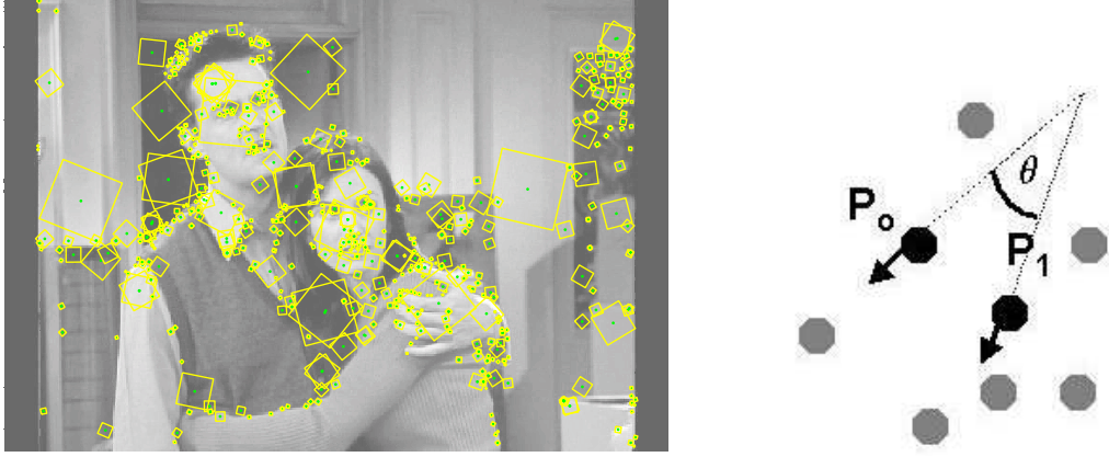
Figure 4: Left : Natural images often contain many partially overlapping distinctive invariant features, which causes their distribution of features to inherently encode information about the spatial configurations of features within local neighborhoods. Detected SIFT features are shown here. Right : For non-overlapping patches, features at the nearest interest points are used to encode spatial constraints.
