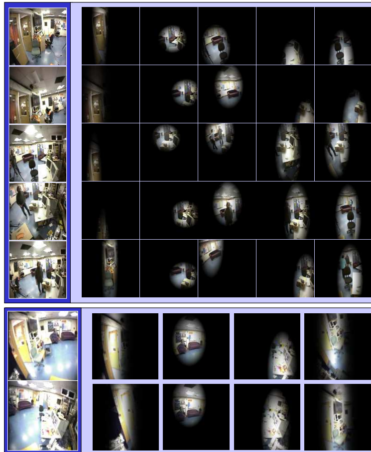
Figure 6.8: Localizing and recognizing objects from contextual cues (Top) Samples of scene images are shown on the first column. The next four columns show probable locations based on context for finding the door, the smaller sofa, the bigger sofa, the table and the chair, respectively. Notice that, even if the object is not visible or present, the system estimates the places at which there is a high probability of finding such an object. Two such examples are shown for the black chair. It also shows that occlusion by humans does not significantly change the context. (Bottom) Results for the scene in Cog's lab for a different day. The training data did not contain any data samples acquired on this day.
