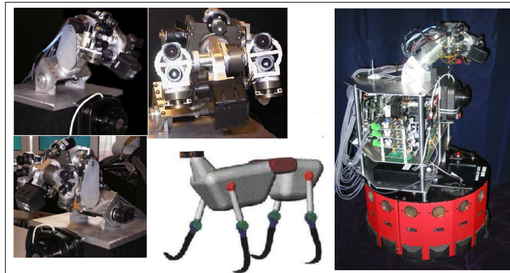
Figure A.2: The M4 Macaco robot, a biologically inspired active vision head designed to resemble a dog's head. It is also shown the original robotic body, resembling a dog, designed and built by the MIT AI LegLab. The head was latter assembled to a iRobot mobile platform, also shown.
