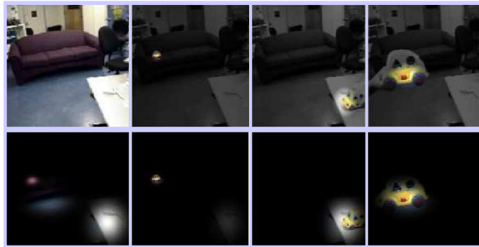
Figure 8.7: The left column shows regions of the image with high probability of finding the car (any size). The next three columns show the regions of higher probability to find the car at a given size scale (smaller, medium and large scales, counting from the left).
