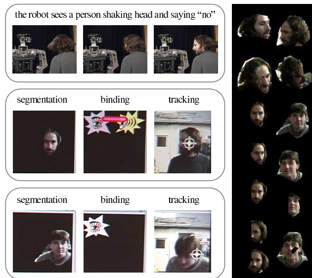
Figure 7.7: In this experiment, the robot sees people shaking their head. In the top row, the person says “no, no, no” in time with his head-shake. The middle row shows the recorded state of the robot during this event – it binds the visually tracked face with the sound spoken. The lower row shows the state during a control experiment, when a person is just nodding and not saying anything. Recorded segmentations for these experiments are shown on the right.
