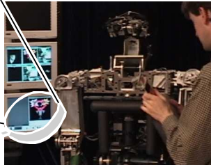
Figure 7.11: In this experiment, a person shakes Cog's arm in front of its face. What the robot hears and sees has the same rhythm as its own motion, so the robot's internal sense of its arm moving is bound to the sound of that motion and the appearance of the arm.
