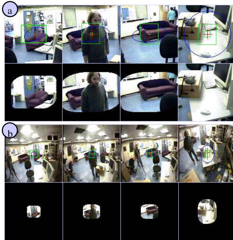
Figure 8.5: (a) Priming object locations. Sample regions (foveal coordinates) computed from predicted size (ellipse) and location (rectangle), plus uncertainties, for objects in a scene. (b) Mapping views. All the data concerning object properties, such as retinal size and location, is mapped onto wide field of view image coordinates, to train the contextual priming system described in chapter 6.
