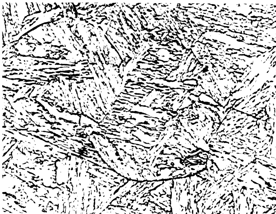
(a) Optical micrograph 1% Nital etch. 1000X
