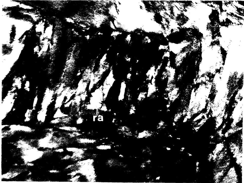
(c) Tempered at 100°C, retained austenite (ra), 15000X.
