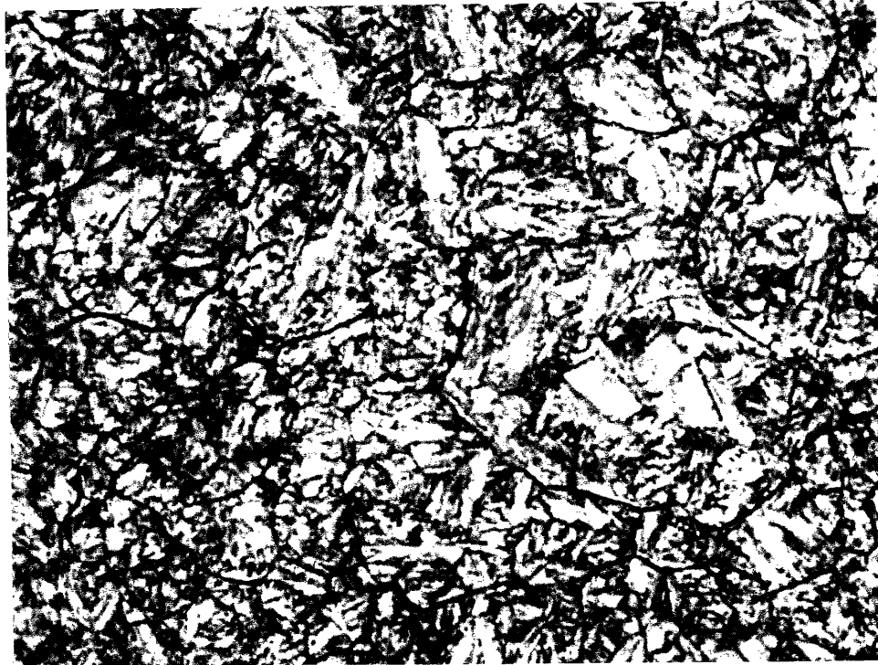
(b) 18Ni-0.4C Twinned Martensite. 1000X
