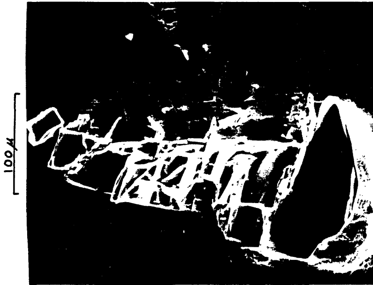
Fig. 32 Annealed Modified 1010 Steel, 800 feet/sec.
