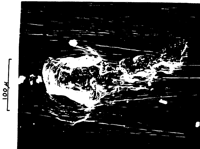
Fig. 20 CR 1020 Steel, 500 feet/sec.
