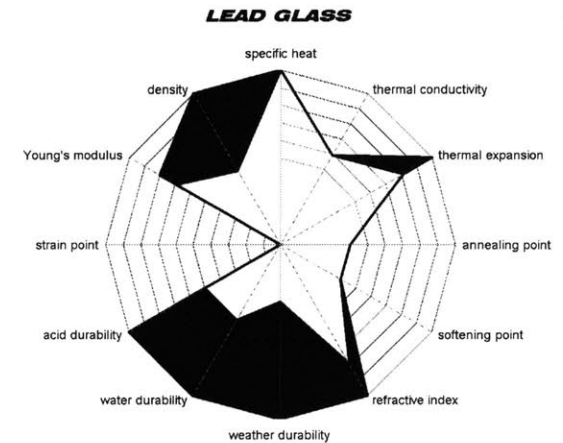
property profile plotted for lead glass illustrating the ranges of values possible within the material family
