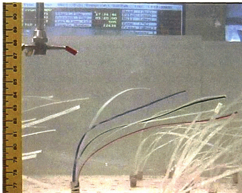
(b) The experimental configuration used to simultaneously measure the flow velocity and plant motion. The heights of three colored blades on one plant were monitored through the capture of digital video and subsequent image analysis. The ADV probe was positioned approximately 3 cm upstream from the front of the plant. The corresponding time in the velocity record (505 s in this case) was clearly visible in each frame.
