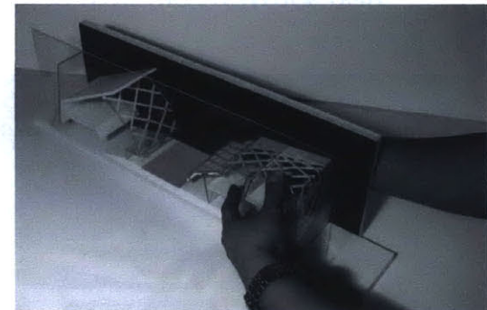
The thermochromic impressions were made by propping the sample securely against the section models. They were heated with a halogen lamp directed towards the section from the skinny end, and cooled by pointing the model towards a cold window.
