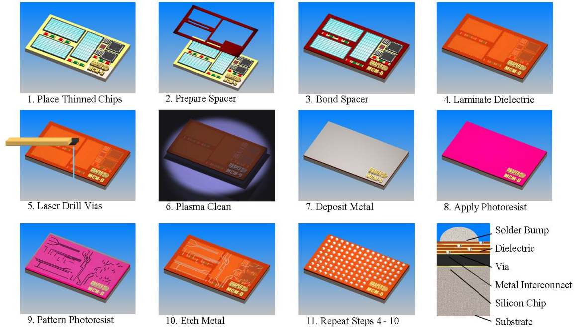
Figure 6-2: Diagram of Draper MCM-D process [15]
