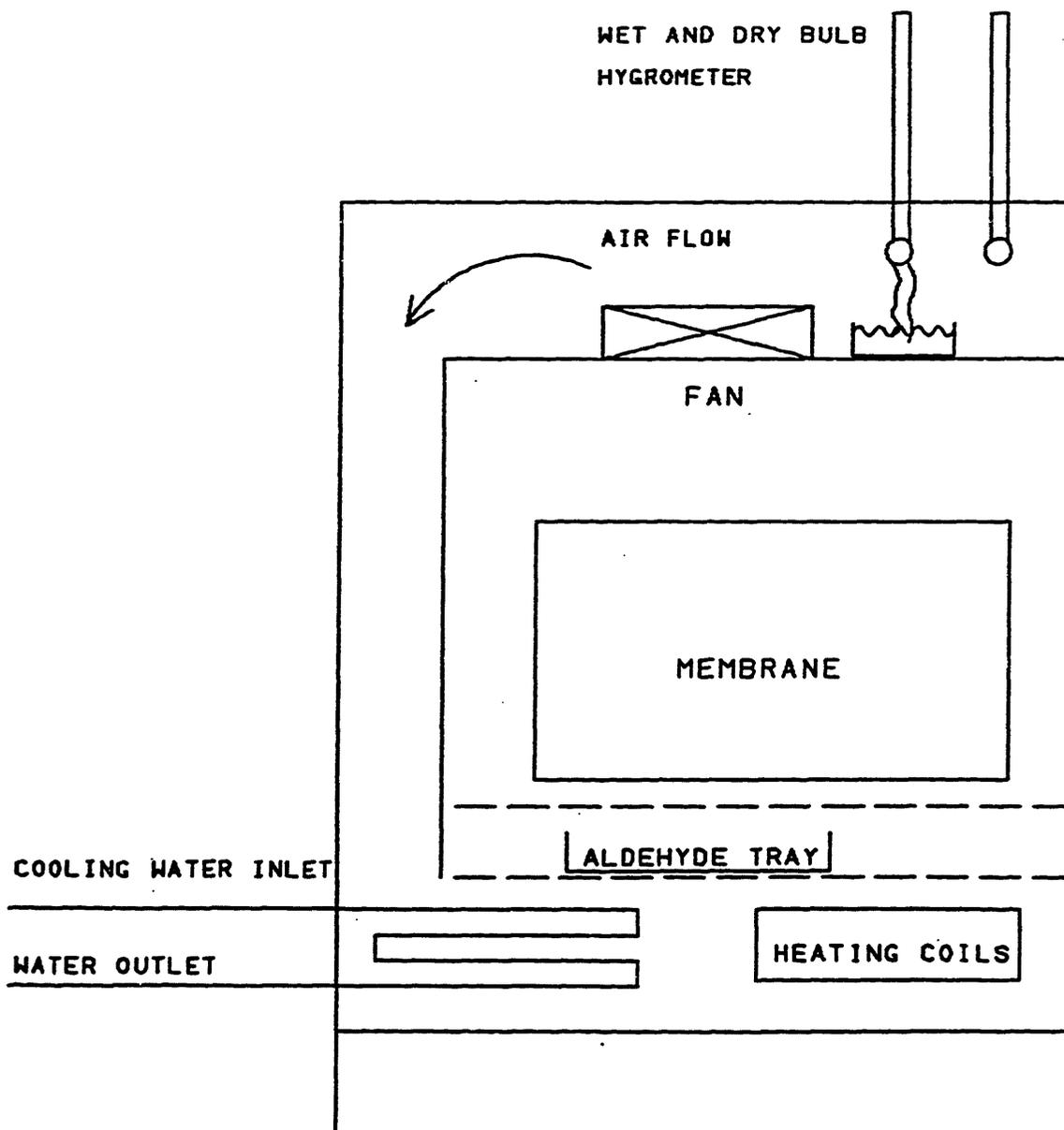
**FIGURE 1.** Schematic of the vapor reactor. The hygrometer was efficiently stirred by the fan. Air flow over the cooling coil and the heating coils provided uniform temperature in the reactor. This air then passed over the aldehyde tray and the membrane to complete the circulation loop.
