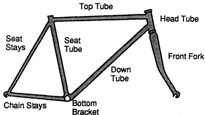
**Figure 4-1: Schematic of a Traditional Bicycle Frame.**
