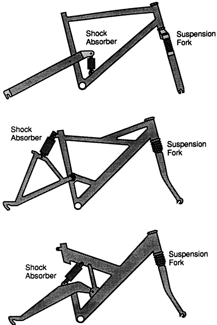
**Figure 4-2: Schematics of Modern All-Terrain Bicycle Frames.** Top design is similar to a frame by Trek Bicycle Corporation. Bottom two designs are similar to frames by Cannondale Corporation.
