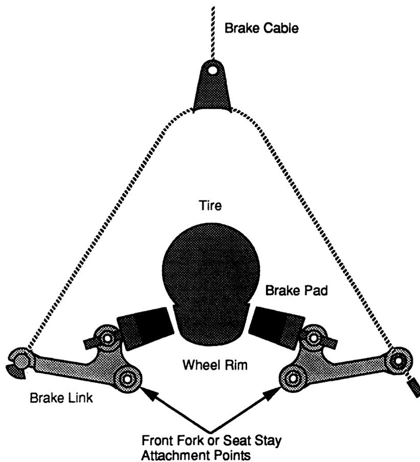
**Figure 4-3: Schematic of a Cantilever Rim Brake.**
