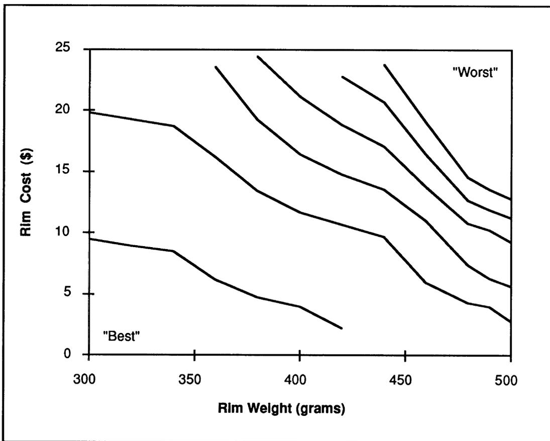
**Figure 5-6: Wheel Rim Weight—Cost Multi-Attribute Utility Contour Plot for Sun Metal Products, Inc.**
