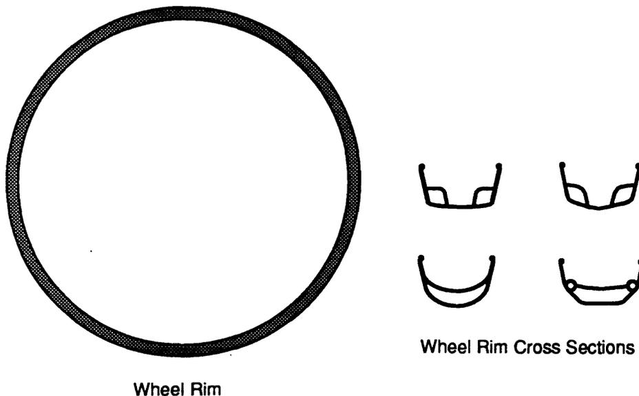
**Figure 4-5: Schematics of a Wheel Rim and of Wheel Rim Cross Sections.**
