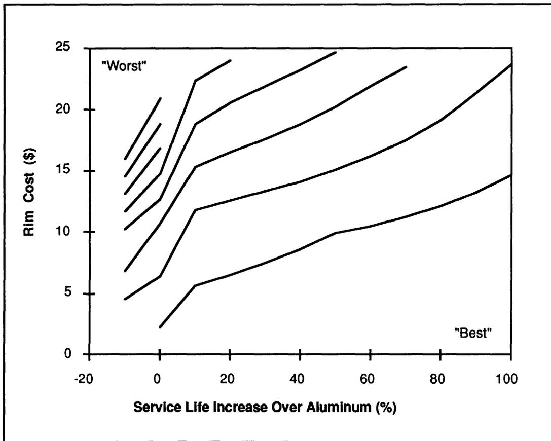
**Figure 5-7: Wheel Rim Service Life—Cost Multi-Attribute Utility Contour Plot for Sun Metal Products, Inc.**
