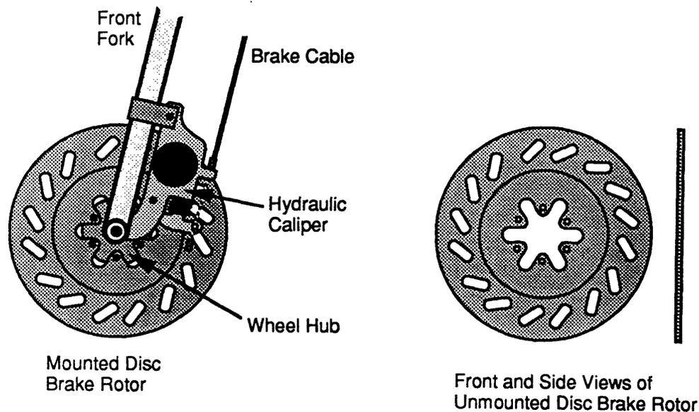
**Figure 4-4: Schematic of a Hydraulically Actuated Disc Brake.** Design is similar to a brake by Dia-Compe USA. The wheel spokes are not shown but connect to the wheel hub behind the disc brake rotor.
