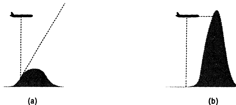
Figure 3-24 Illustration detection errors. In (a), alert logic based on terrain closure rate produces false alarms, opposed to missed detections in (b) (based on Kuchar & Hansman [78])
