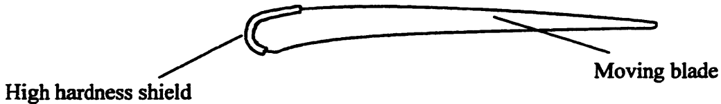
Figure 5.21. Erosion shield on a moving blade (from [Beaudry 1992]).
