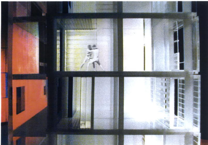
Section through model showing single-loaded corridor and stacked units
