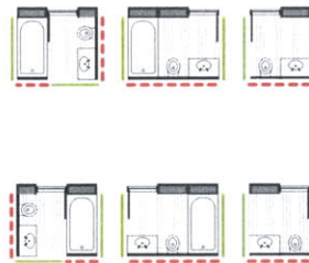
Bathroom group wet wall adjacencies (dashed red line) and enclosure (solid green line).
