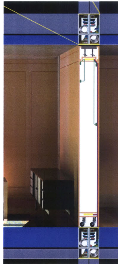
Section detail of infill and volumetric chassis connection. Image by T. Lawrence
