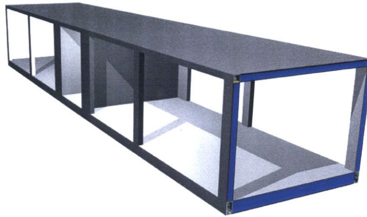
Volumetric chassis modules designed to be thirteen feet by sixty-four feet in dimension, so that two modules side-by-side fit precisely over the parking column grid. This is approximately the maximum size object that can be efficiently carried over the highway (thirteen feet wide by sixty-four feet long).
