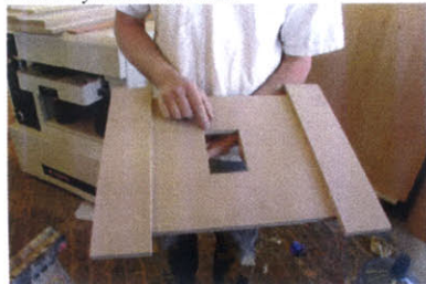
A jig produced for implementing the detail. Photo by Ron MacNeil.
