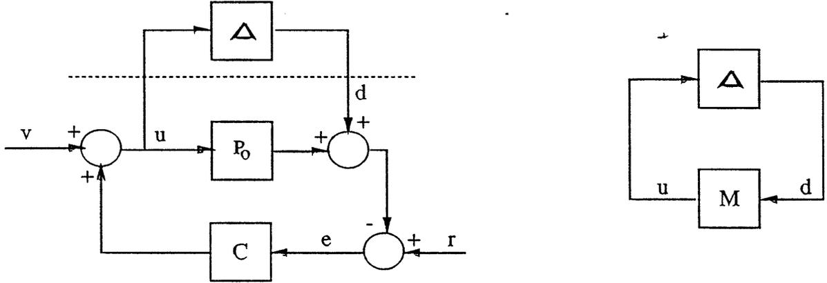
Figure 3: Transformation to Small Gain Loop
