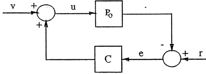
Figure 2: Centralized Two Block Problem
