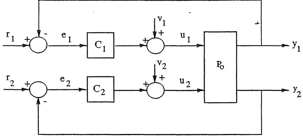
Figure 1: The Two Channel Decentralized Control Problem
