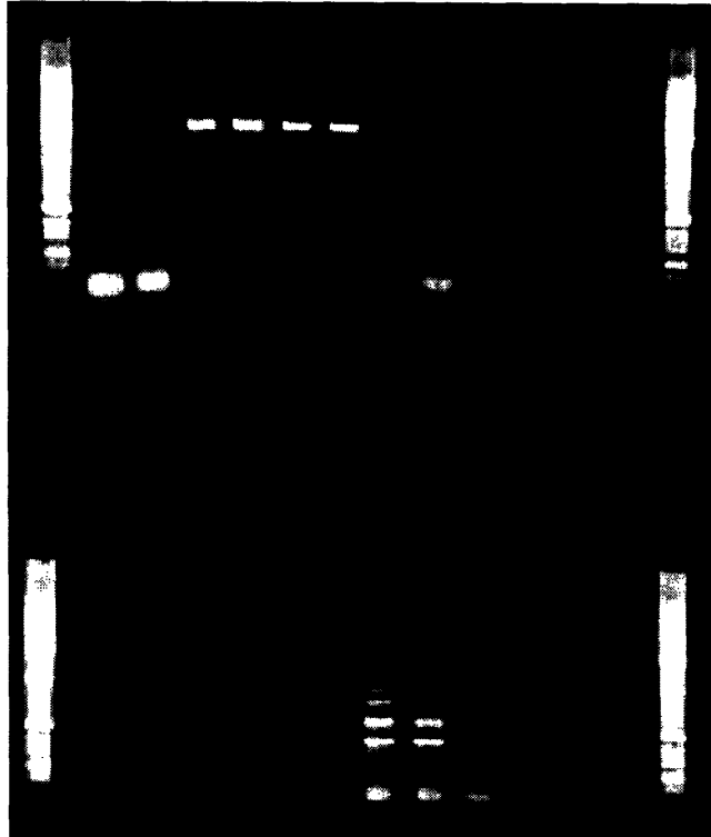
Figure 3-1: Gel electrophoresis analysis of PCR reactions used to amplify DNA sequences for creating microarray printing stocks. Each quadrant of the gel contains one lane of a 1-kb DNA ladder standard and six lanes of samples from PCR reactions used to amplify one particular sequence. Each of these six reactions was carried out at a different annealing temperature—54.0, 55.5, 57.0, 58.5, 60.0, and 62.5 °C from left to right. The lowest bands in each lane consist of unincorporated material.
