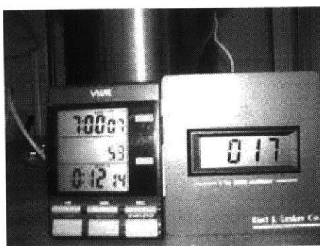
Figure 4.20: The vacuum gage displaying the vacuum pressure with timer showing the time to reach that pressure.
