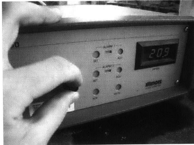
Figure 4.18: The oxygenmeter calibration process.
