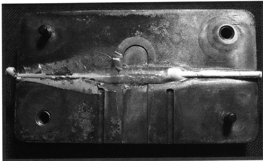
Figure 24. Gas bubbles form if the melt is too hot (example: hot temperatures cause insulation damage and bubbles in the cavity).
