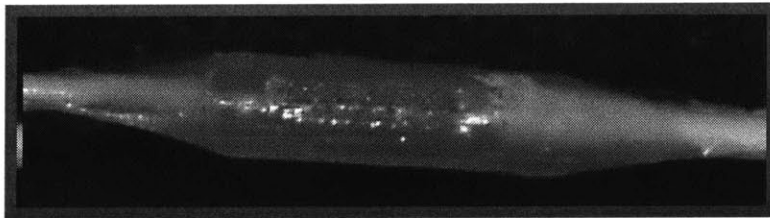
Figure 25. A finished splice (the smaller wire, 26 AWG, is shown on the left and the larger wire, 20 AWG, is shown on the right).
