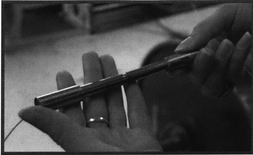
Figure 11. A “mold insert” used in the SCD machine. Custom mold inserts, that fit in the SCD machine, assist in the development of an optimal cavity profile (designating the coating’s shape). (See Appendix B.4 for part drawings of mold inserts designed for this project.)
