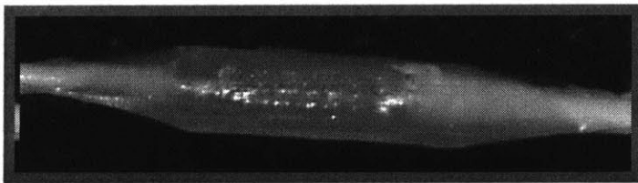
Figure 9: A molded coating around an ultrasonically welded wire connection. (This photograph was taken of a sample made later on into this project.)
