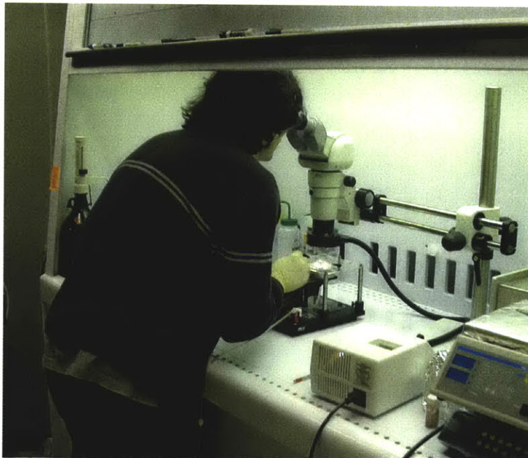
Figure4–9: Alignment for PDMS bonding or packaging is carried out in the fume hood to reduce particulate contamination.
