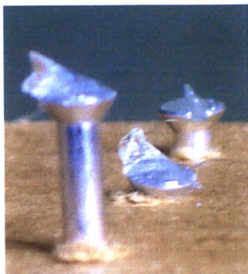
Figure 4. 9: Photograph of the nanocomposite thin-film fixed with epoxy upon a cryotome post.
