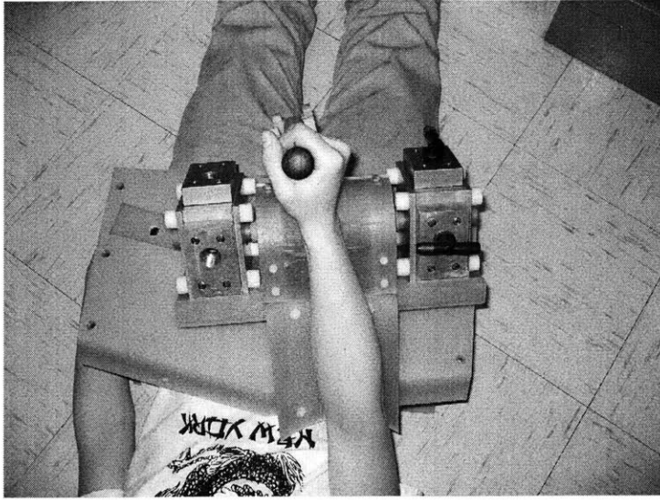
Figure 7-4: A patient inside the MRI compatible wrist robot
