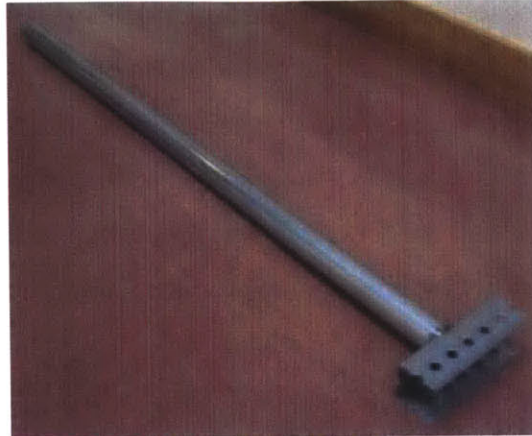
Figure 7-46: Welded Upright for Prototype Railing
