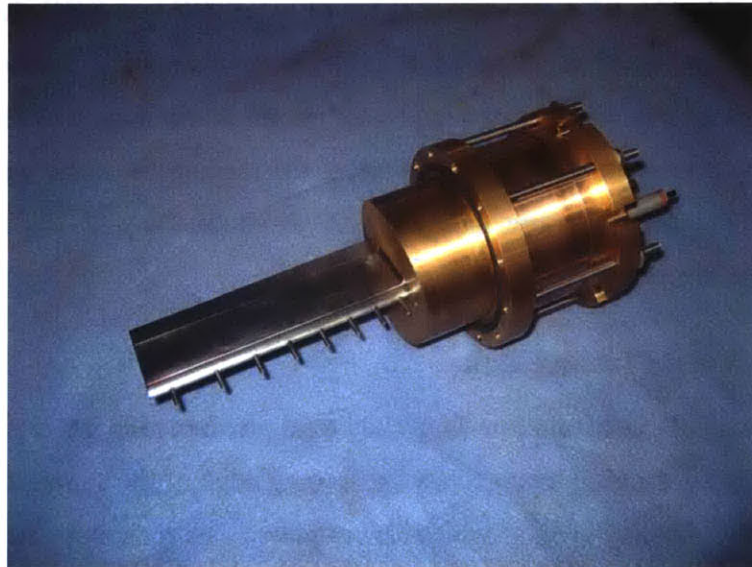
Figure 4.1 – Fully-Assembled Upstream Total Pressure Rake.
