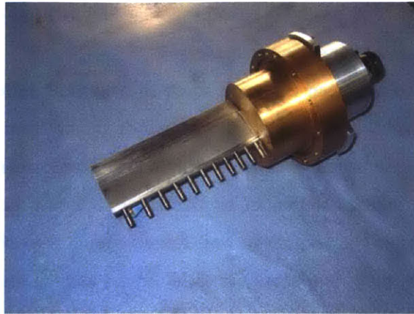
Figure 3.7 – Fully assembled upstream total temperature rake.
