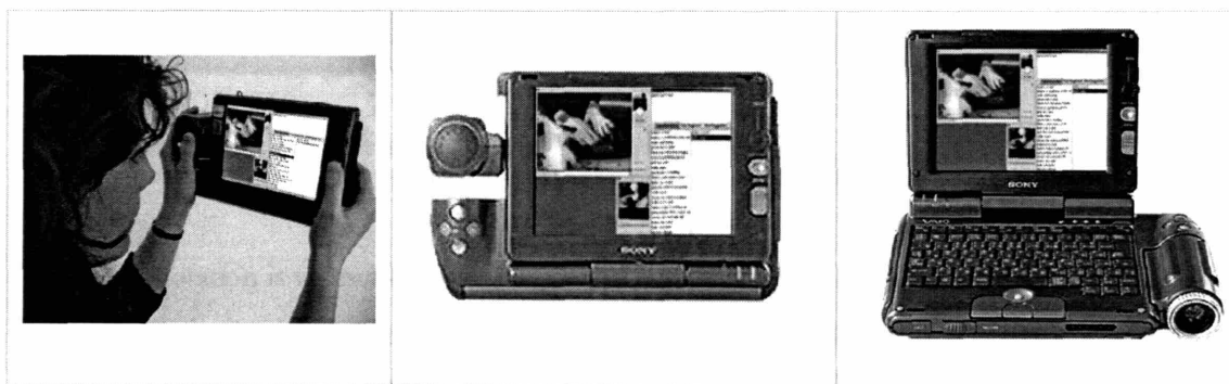
Figure 7: The camera platform running the mindful camera and video recording software. The picture on the left shows the camera being used in recording position. The picture in the middle shows the camera in recording position. The screen is turned and lies flat across the keyboard and the lens turns. The picture on the right shows the camera platform in the position for typing annotation and selecting suggestions. After each shot the videographer twists the screen from recording position to the open laptop position in order to type and select suggestions, then turns it back to recording position to shoot.
