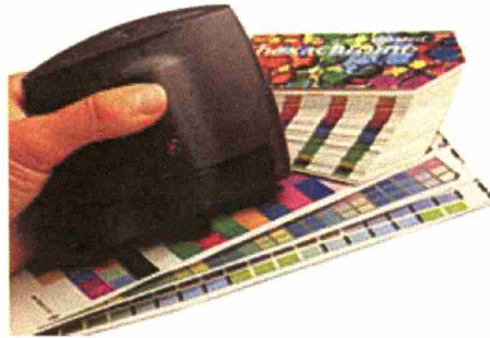
Colortron™ is a spectrometer for designers to work with precise color values.
