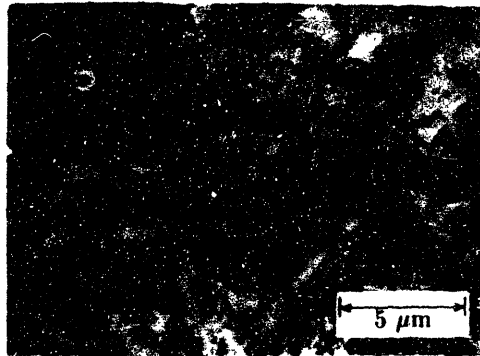
Figure 5.1: Bright-field micrographs of films implanted at 5 \times 10^{15} ions/cm 2 and annealed at 630°C for three anneal times: (a) 4 hours, (b) 5.25 hours, and (c) 7.1 hours. Diffraction patterns are inset.
