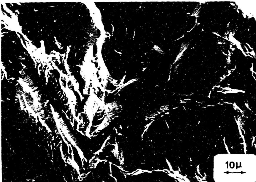
Figure 4.41 Typical transgranular fracture surface features for Inconel 718 tested at 427C under elastic fatigue conditions.
