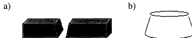
Figure 11: a) V-shaped taper: created when cutting at high speeds. b) Sweeping out of arcs: caused by high speed cutting around an arc resulting in a cone shape
