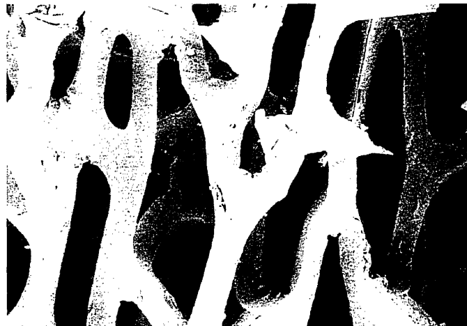
Figure 5 Scanning Electron Micrograph (SEM) image of a cut surface of polyurethane foam under 45 % strain (Lee, 1997)
