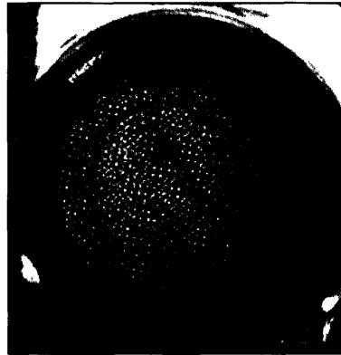
Figure 10: Infrared-illuminated chamber, viewed with an USB2 Orange Micro iBOT camera [21]. The large circle in the center is an air bubble and the dark line on the right is the planaria.
