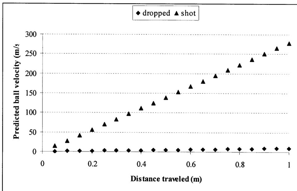
Figure 21. Predicted ball velocity from dropping ball and shooting it with fully-compressed pinball shooter. Drag is neglected. Slope of each data set is the acceleration.
