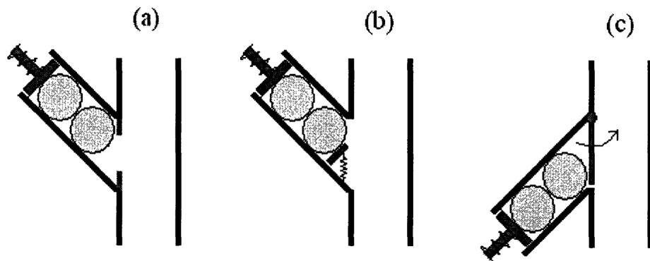
Figure 14. Possible spring-loaded piston loading mechanisms: (a) rubber annulus, (b) spring-loaded plate, and (c) hinged flap.
