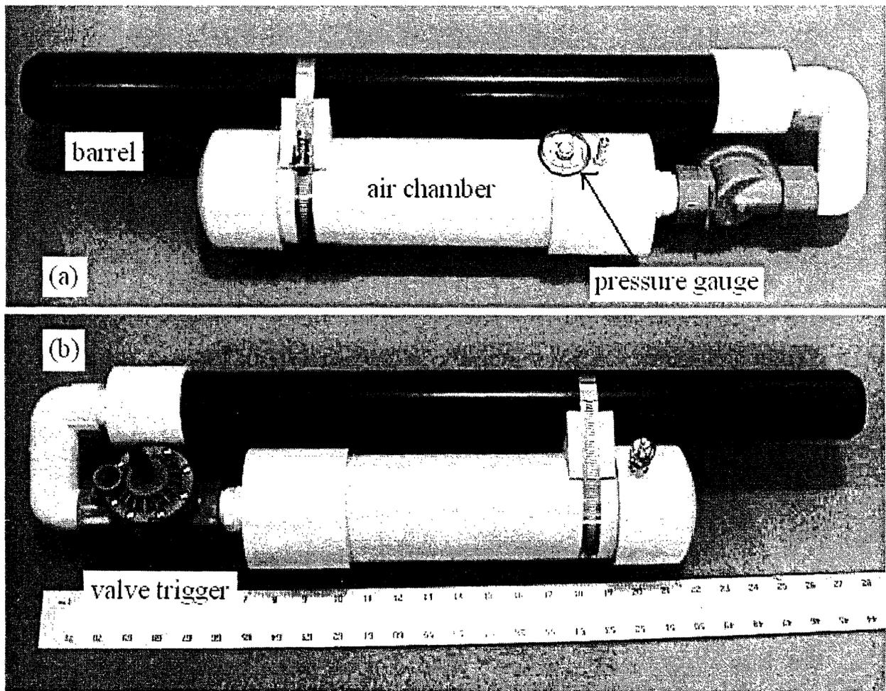
Figure 5. Two views of simple potato shooter. (a) Pressure gauge monitors pressure in air chamber. (b) Valve trigger allows air to flow from chamber to barrel to shoot potato [13].
