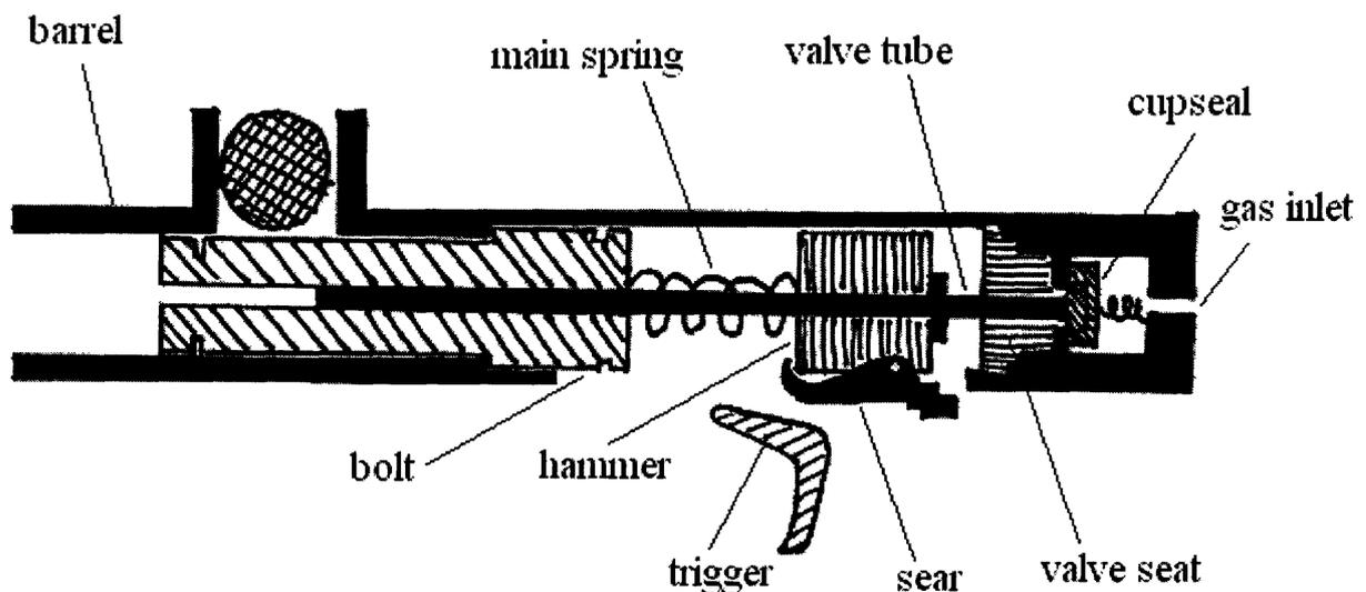
Figure 8. Cross-sectional diagram of simple paintball gun before shooting. Not to scale. Pin attaches sear to hammer. Cupseal is fixed. Valve tube can move freely through bolt, hammer, and valve seat.
