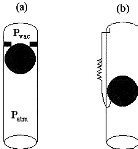
Figure 11. Ideas to hold ball in barrel: (a) suction and (b) spring and hook.
