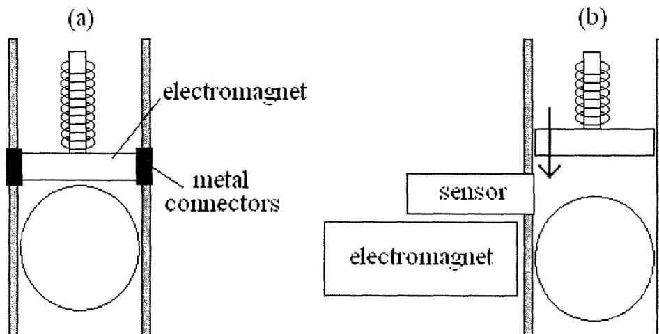
Figure 17. Possible electromagnet locations: (a) integrated in the piston and (b) outside barrel.
