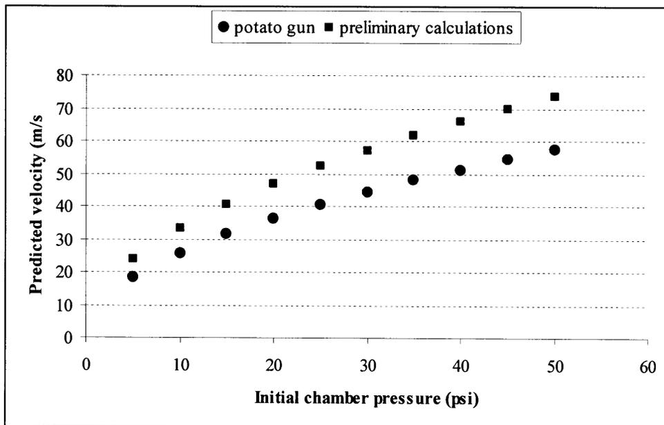
Figure 7. Predicted potato launcher and preliminary calculations muzzle velocities as a function of pressure for barrel diameter = 0.1 m, barrel length = 1 m, projectile mass = 1 kg, no friction, and no dead volume. Volume ratio for potato launcher is 1:1. Pressure is absolute pressure.
