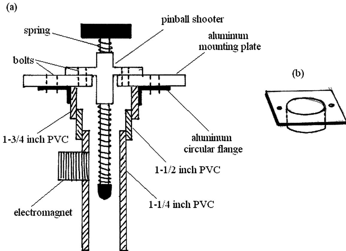
Figure 18. Diagram of final design. Not to scale. (a) Cross-sectional view of entire design. (b) Welded aluminum circular flange.
