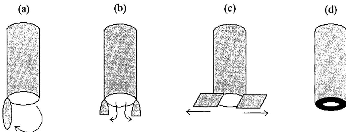
Figure 10. Ideas to hold ball at end of barrel: (a) one hinged flap, (b) two hinged flaps, (c) two sliding plates, and (d) rubber annulus.
