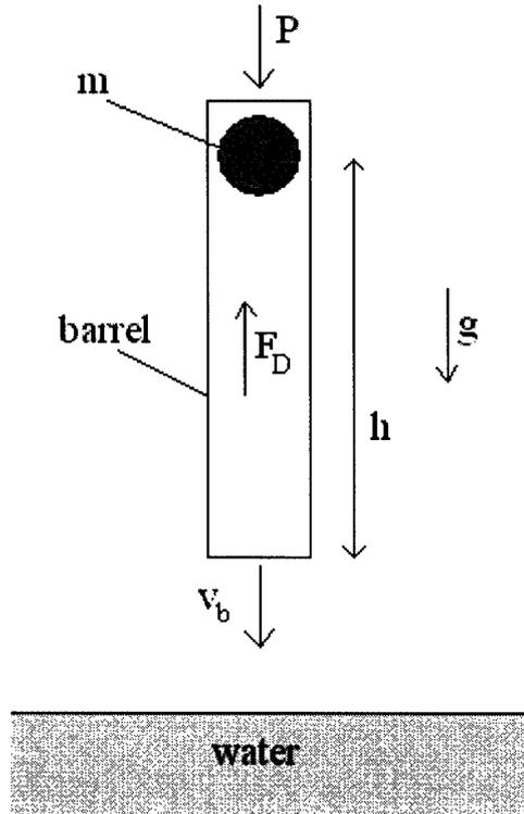
Figure 3. Basic shooting system. Barrel has cross-sectional area  $A$  and height  $h$ . Ball of mass  $m$  is acted on by pressure  $P$ , gravity  $g$ , and a drag force  $F_D$ . Ball exits barrel at velocity  $v_b$ .
