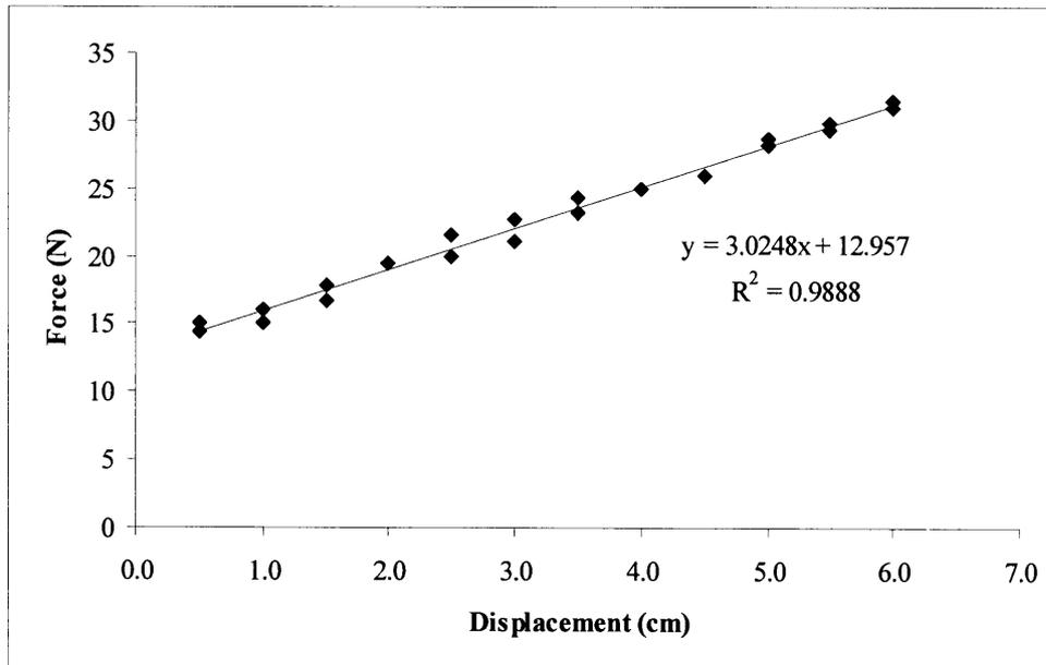
Figure 20. Force as a function of displacement for pinball shooter spring. Spring constant  $k$  is the slope.
