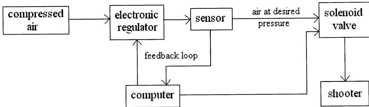
Figure 4. Sample control system. The electronic regulator transmits air from the compressed air source to the rest of the system at the desired pressures. The sensor adds a feedback control loop. The solenoid valve opens when signaled by the computer, transmitting the air to the shooter.
