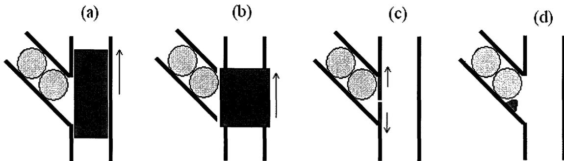
Figure 13. Possible gravitational loading mechanisms: (a) sliding bolt, (b) sliding sleeve, (c) sliding plates, and (d) retractable nub,.
