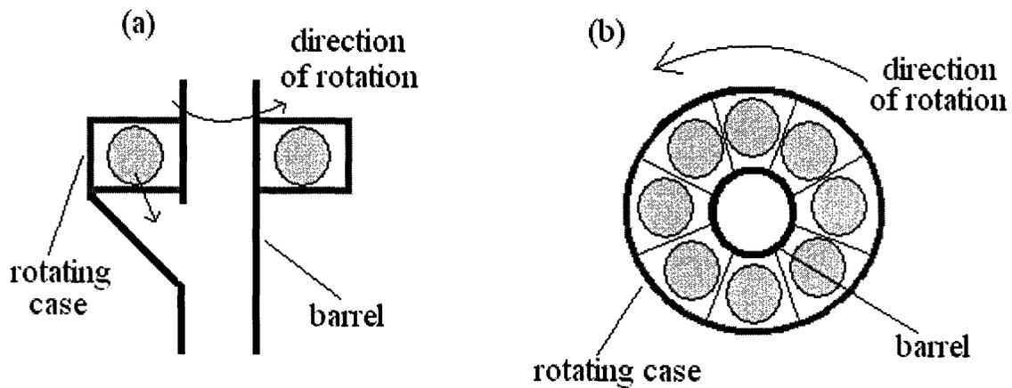
Figure 15. Rotating loading mechanism. (a) Side cross-sectional view. (b) Top view of rotating case.
