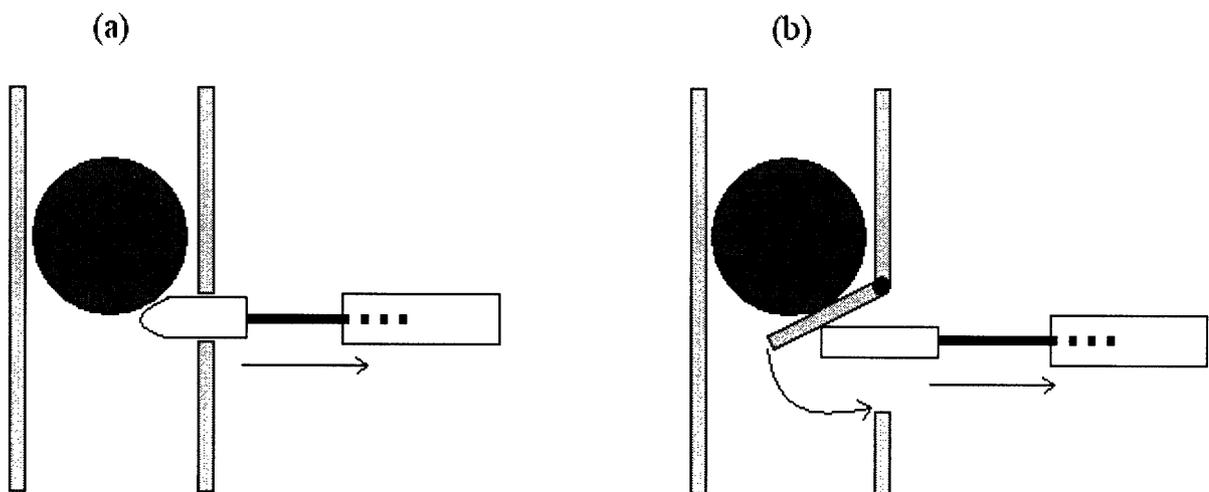
Figure 12. Ideas to hold ball in barrel involving a retractable piston: (a) linear nub and (b) hinged flap.
