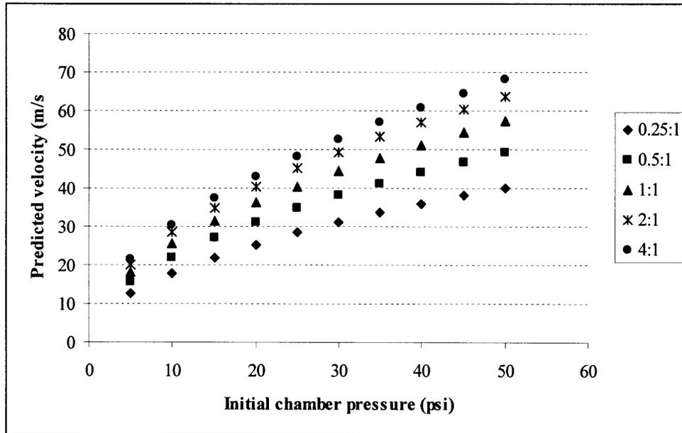
Figure 6. Predicted potato launcher muzzle velocities as a function of initial chamber pressure for barrel diameter = 0.1 m, barrel length = 1 m, projectile mass = 1 kg, no friction, and no dead volume. Volume ratios are ratios of chamber volume to barrel volume. Pressure is absolute pressure.
