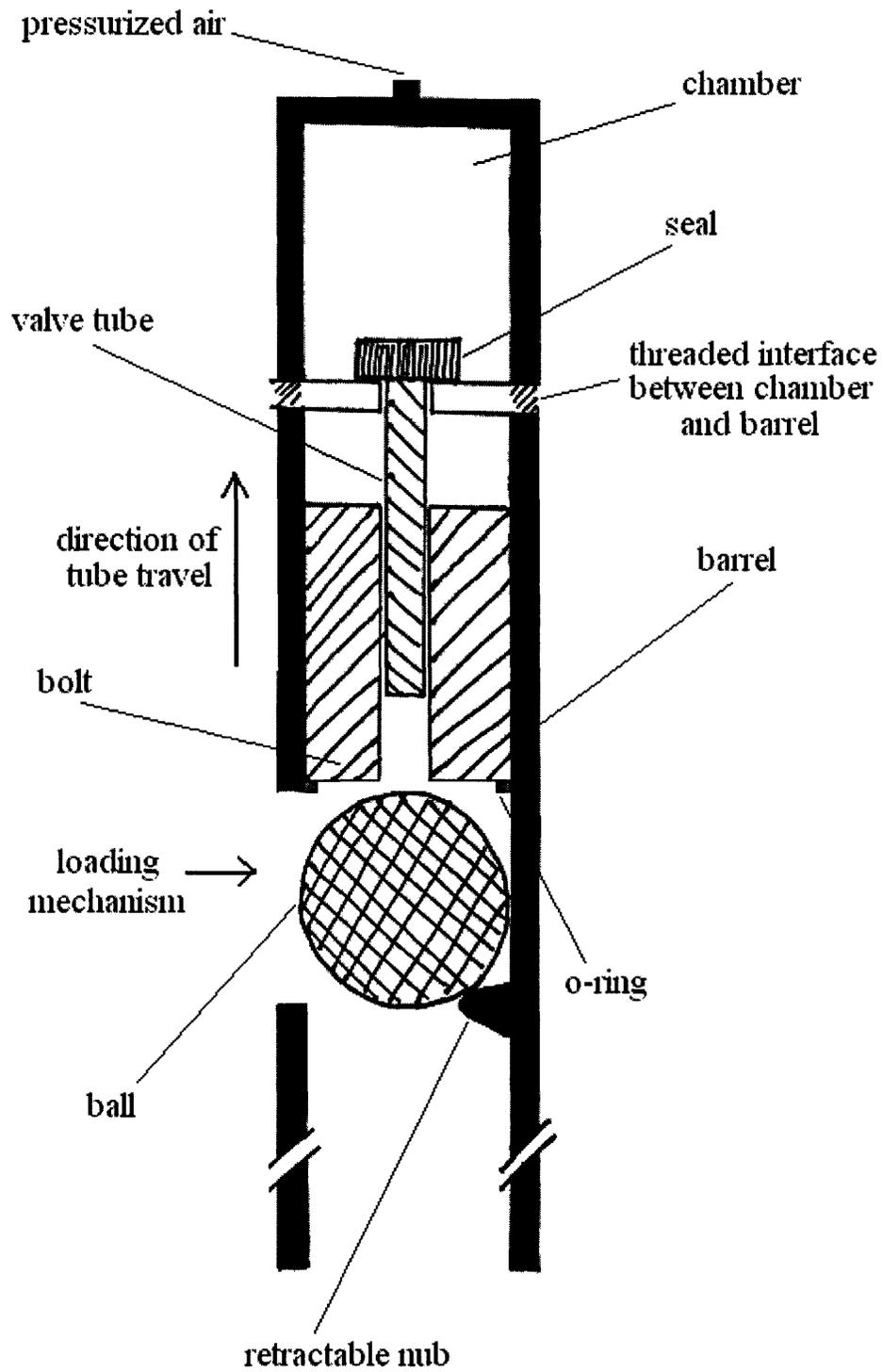
Figure 9. Cross-sectional diagram of paintball gun adaptation. Not to scale. Bolt is fixed in barrel. Loading mechanism and retractable nub discussed later.
