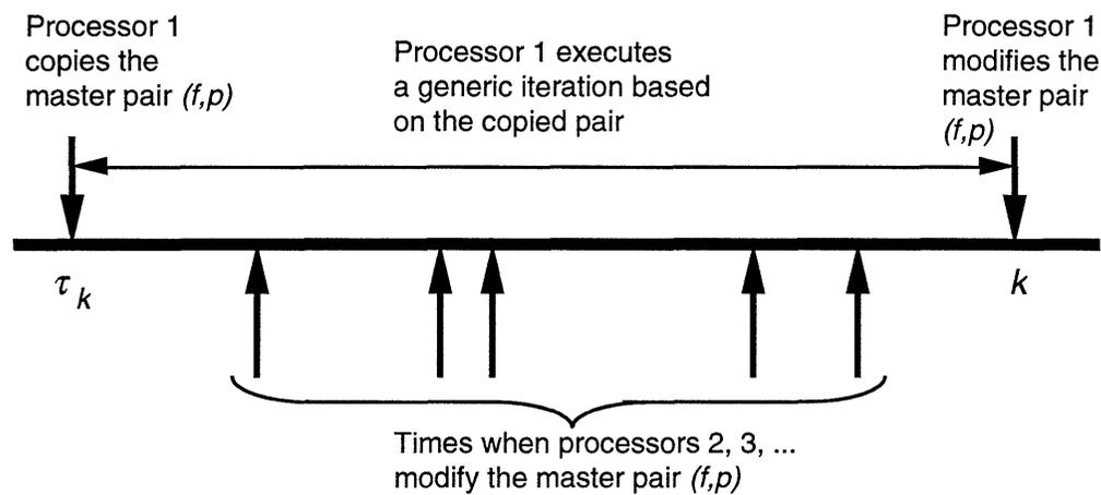
**Figure 1:** Operation of the asynchronous algorithm in a shared memory machine. A processor copies the master flow-price pair at time  $\tau_k$ , executes between times  $\tau_k$  and  $k$  a generic iteration using the copy, and modifies accordingly the master flow-price pair at time  $k$ . Other processors may have modified unpredictably the master pair between times  $\tau_k$  and  $k$ .
