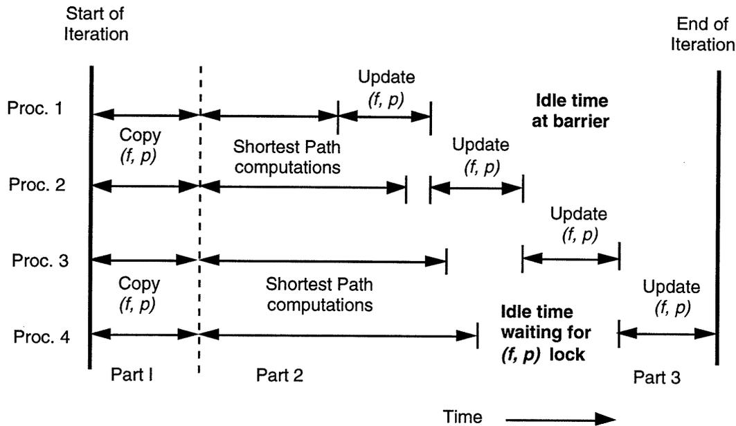
**Figure 2:** Timing diagram of an iteration. The computation of each processor consists of three parts, possibly separated by idle time. In the first part, all processors copy (in parallel) the master pair  $(f, p)$ . In the second part, the processors calculate (in parallel) their shortest augmenting paths. In the third part, the processors update (one-at-a-time) the master pair  $(f, p)$ . The next iteration does not begin until all processors have finished all three parts.
