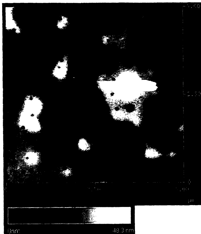
Figure A.1: PS(16.5)-b-PAA(4.5) with FeCl 3 on PEM. 5 μm scale with a scan rate of 1 Hz. Craters are spread throughout film. Maximum height = 40.38 nm.
