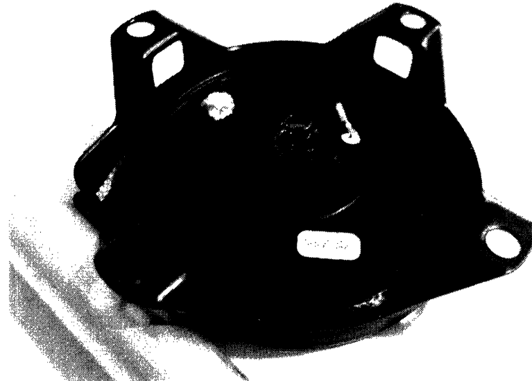
Figure 5: The recoil mechanism is pictured with black casing and inner pulley and spring. The aluminum tube handle bar is also attached.
