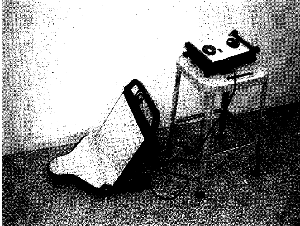
Figure 1: On the right, the Kinkajou projector is pictured. The Kinkajou uses a 6W LED and can be used to teach literacy classes during the evening and night. The Kinkajou human powered generator is pictured on the left and is attached to the kinkajou projector that it powers.
