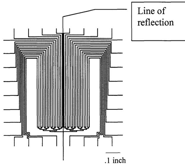
**Figure 3.2:** Diagram of the pattern used to create the cell channels and the line about which the design is mirrored.
