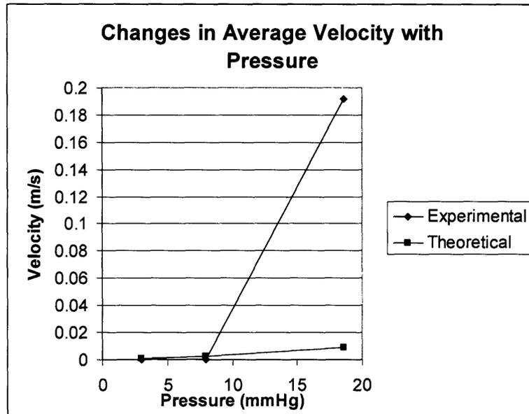
**Figure 6.1:** Theoretical versus Experimental average velocity at different pressures.
