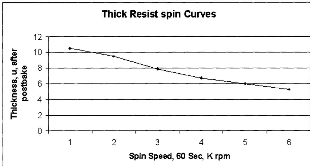
**Figure A.1:** Spin curve of thickness of AZ4620 for a 60 second spin coat [18].
