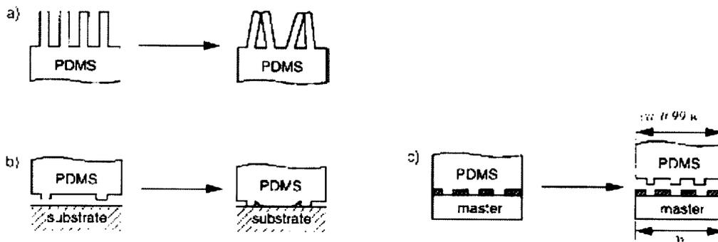
**Figure 3.4:** Possible problems of design transfer using elastomers. A) Pairing. B) Sagging. C) Shrinking. [8]
