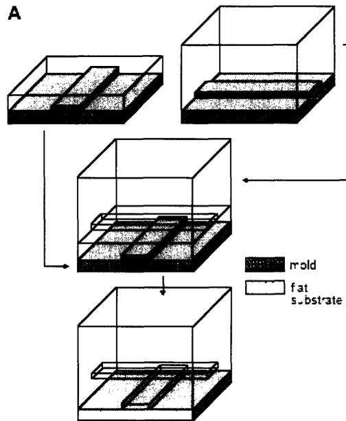
**Figure 3.7:** Diagram showing steps used to create a multilayer elastomer valve. The two channels are stacked perpendicular to each other creating a thin membrane between the two channels that acts as a valve.
