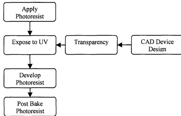
**Figure 4.2:** Steps to create a master mold using photolithography.
