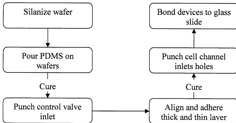
**Figure 5.1:** Process for fabrication of PDMS device with multilayer elastomer valves.
