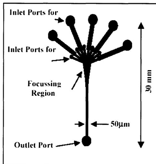
**Figure 2.1:** Liquid phase microreactor with focusing region, Floyd *et al.* [4].
