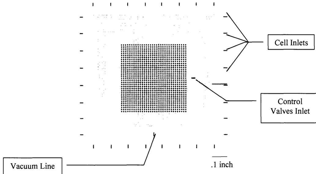
**Figure 3.1:** Layout of cell channels and control valves and location of bored holes for inlets and the vacuum line.
