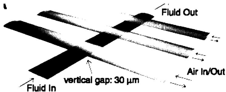
**Figure 3.6:** Scale diagram of a monolithic multilayer elastomer valve system
