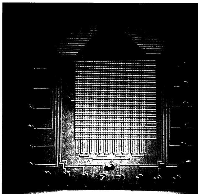
**Figure 5.2:** Final device sealed to a PDMS coated glass slide with valves open.
