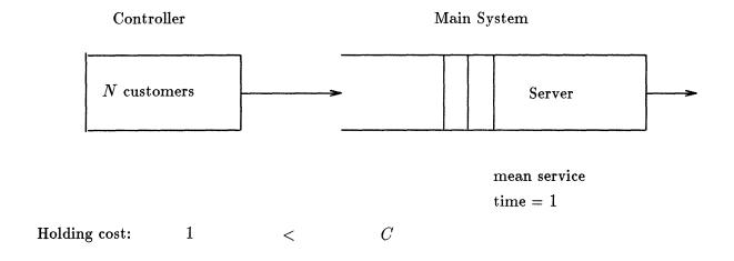
Figure 1: A system consisting of a controller followed by a single server queue
