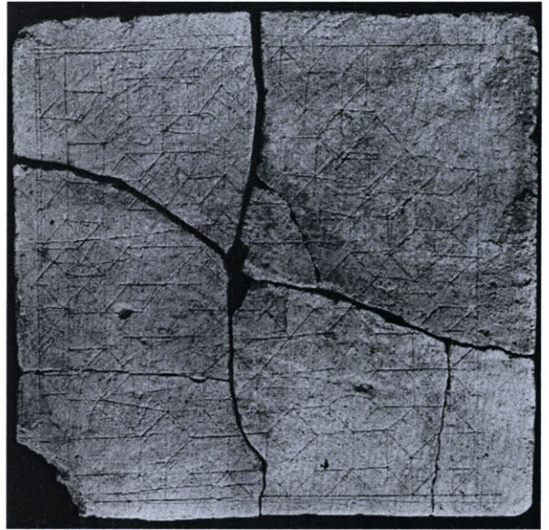
Fig. 22. The earliest example of a full-scale muqarnas drawing etched on a plaster slab.
