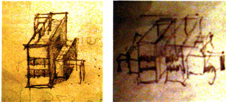
Figure 6. Examples of early sketches, depicting a possible house unit (left), and use of symmetry transformations for its placement in a given lot (right).
