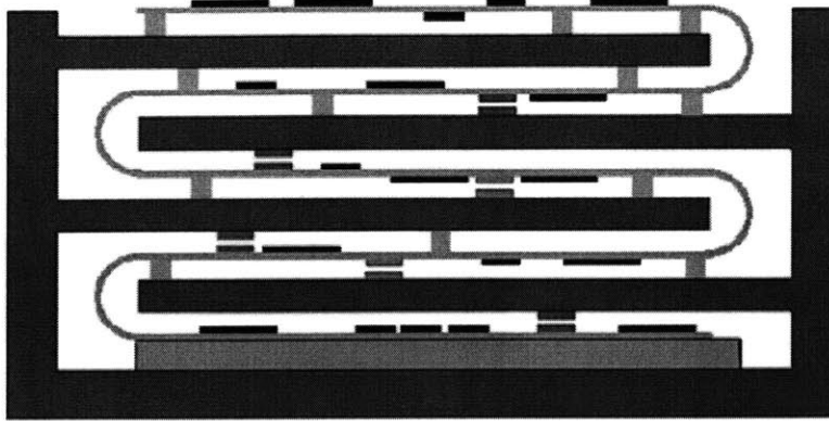
Figure 1-2: Folding a pre-patterned membrane into a 3-D configuration will maximize the possible interconnections and make best use of available space.
