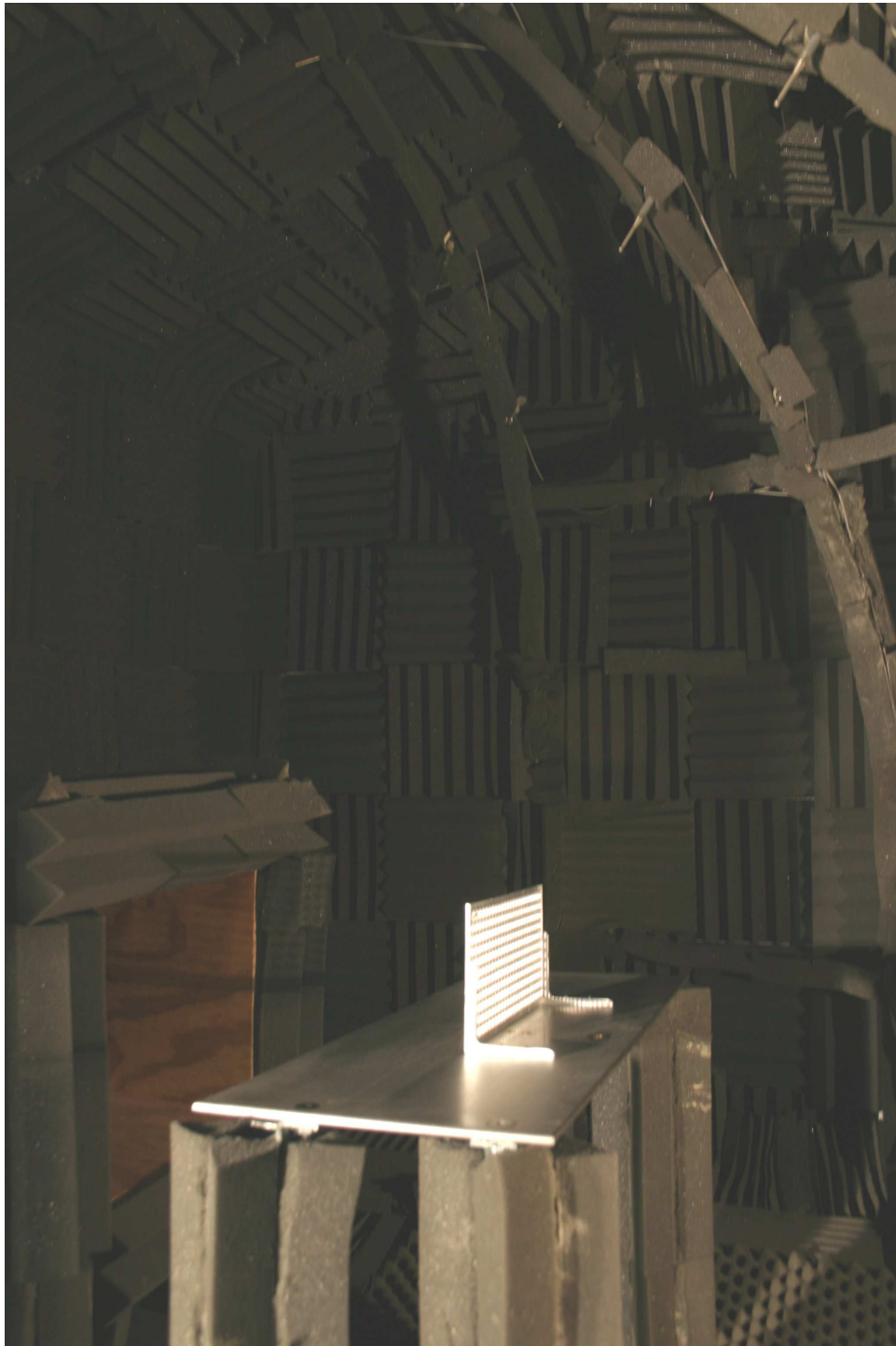
Figure 4-1: Perforated plate with \beta = 60\% porosity mounted in a spoiler configuration.
