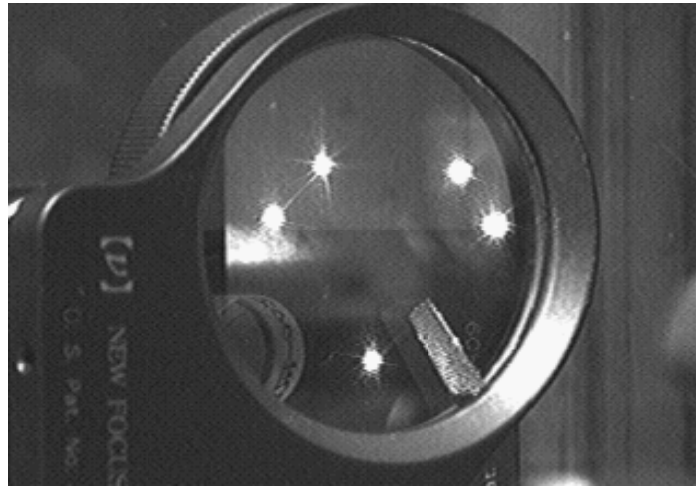
Figure 2.2: 5 reflections per each mirror in a 15 MHz laser are shown in a single path.
