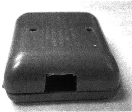
Figure E.17: Notch and holes on casing
