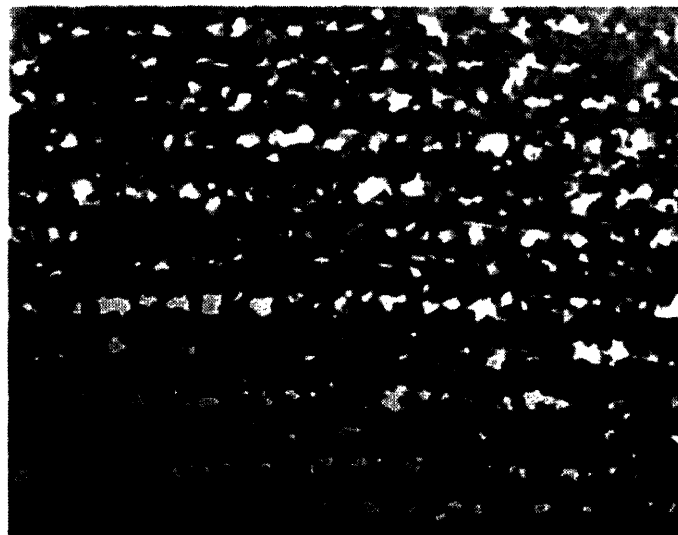
Figure 11.4 The second roughened structure analyzed with the homogenization approximation [Hsiao (2005), reprinted with permission]. Although it is not apparent to the eye, there are three periodicities built into the structure.
