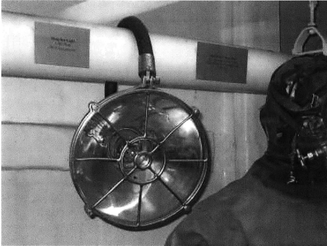
Figure 2-7: This 1000W underwater work light was used by divers during WWII. The light is on display at the Charleston Naval Shipyard Museum on the USS Yorktown, Patriot's Point, Mt. Pleasant, SC. Photo by the author.
