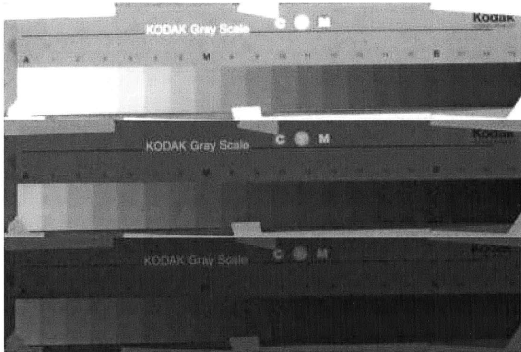
Figure 2-11: Three different images of the same Kodak contrast target. The center image is correctly exposed (note that each step of the bar is visible). The top is overexposed (white and light gray saturate, so both appear white). The bottom is underexposed (black and dark gray do not register, so both appear black).
