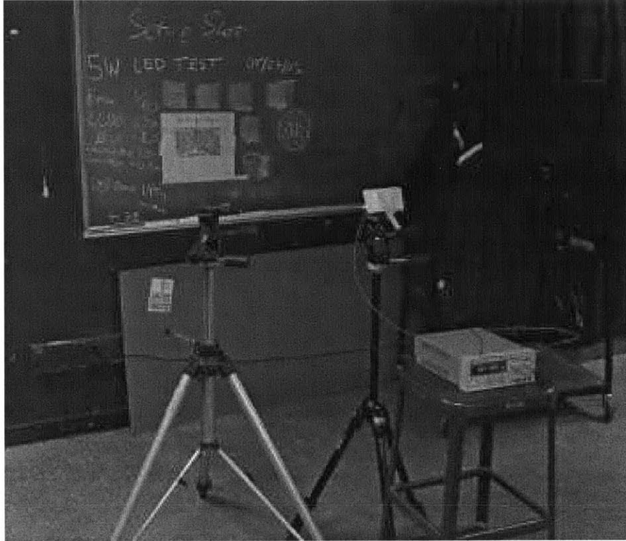
Figure 3-6: The setup of the preliminary LED and camera characterization experiment in the MIT Strobe Lab. The empty tripod in the center of the image holds the camera (when not being used to take this image). The image was taken using ambient fluorescent light in addition to a blue 5W LED to better show the true colors of the target and to allow a hand-held image to be taken.
